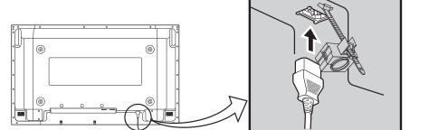
Fix the AC cord plug securely to the Plasma Display with the clamper. (See page 9)
